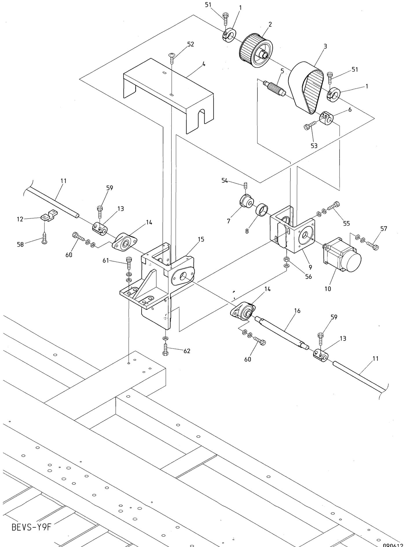
10E Pantograph drive E
